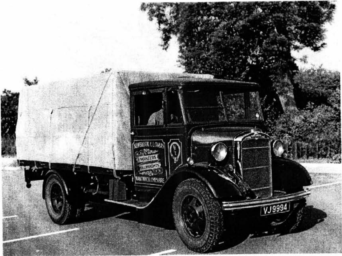
Fig 5: Morris type C with forward control typical of Crowe's patent. Photo Roy Streetton
