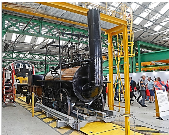
The Greatest Gathering: former S & D R Locomotion No. 1 built by George and Robert Stephenson 1825, the first steam locomotive to use coupling rods.
